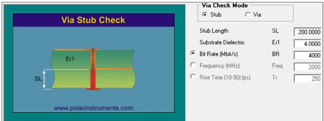
Figure 1: Via stub length of 200 mils requires attention at 4 Gbit/s data rate. Find the math behind this in *Signal and Power Integrity Simplified*, by Dr. Eric Bogatin.
