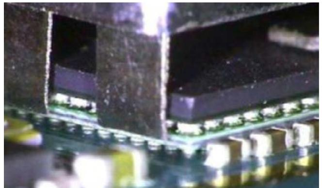
Figure 13: Tweezer nozzle (Finetech) removes both packages together.
