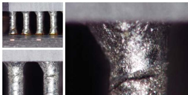
Figure 8: Optical photomicrographs of re-columned and reassembled CGA 560 I/Os after thermal cycles and prior to X-sectioning showing microcracks in columns and solders at the package side.
