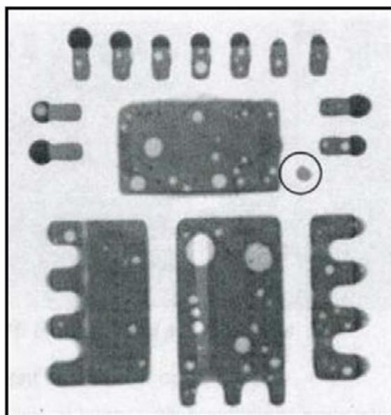
Figure 24: Example of voiding and solder balling under a power QFN<sup>[7]</sup>.
