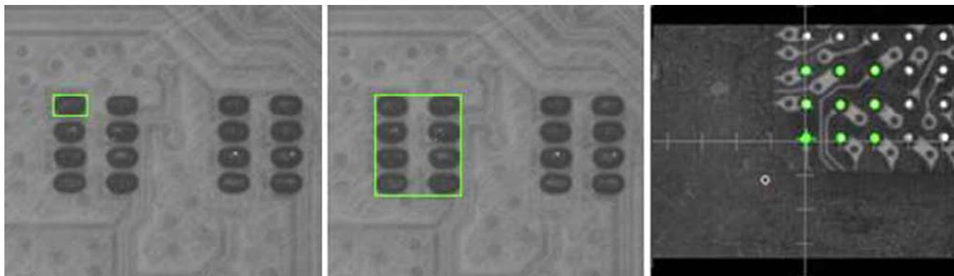
Figure 5: Single and pattern fiducial recognition.
