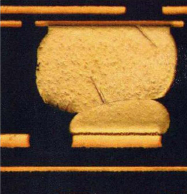
Figure 11: HiP defect<sup>[4]</sup>.
