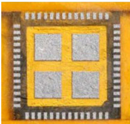
Figure 25a: QFN with stencil and solder paste<sup>[8]</sup>.
