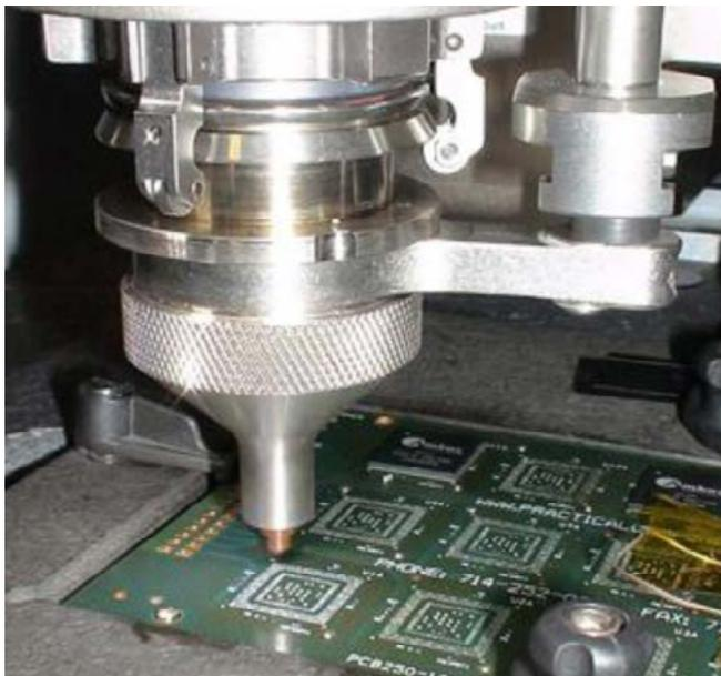
Figure 14: Non-contact site cleaning system.
