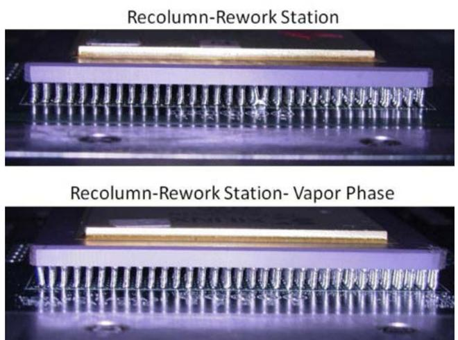
Figure 5: Representative of optical photomicrographs for re-columned 560 I/O package assemblies.
