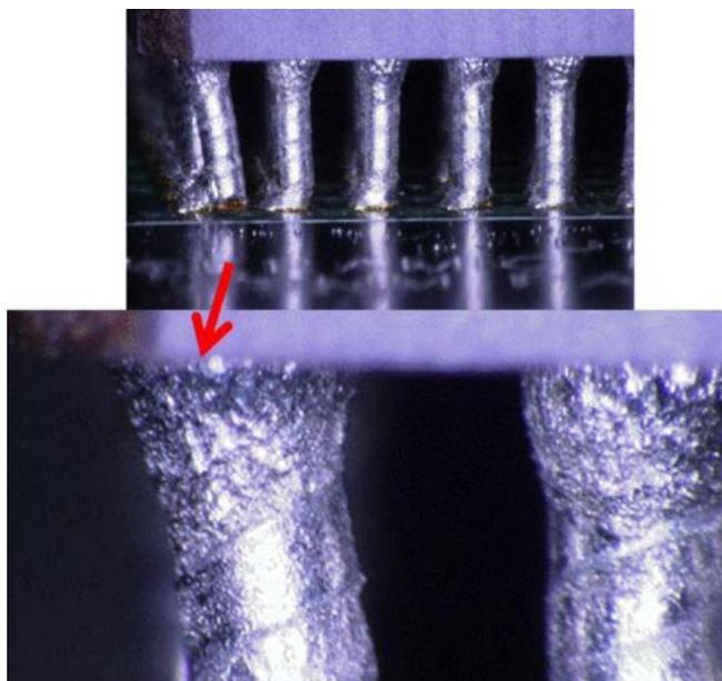
Figure 7: Optical photomicrograph re-columned and reassembled CGA 560 I/Os after thermal cycles showing microcracks in solder at the package side.
