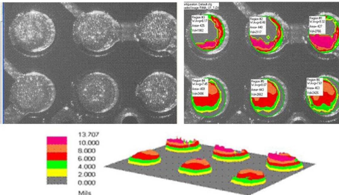
Figure 17: Optical photomicrograph and measured/calculate paste information for paste print with ministencil with 8-mil thickness and 28-mil aperture opening diameter.
