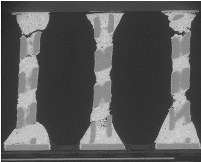
Figure 11: X-section photomicrographs of re-columned and reassembled CGA560 after thermal cycling showing microcracks and separation mostly at the package side (top).
