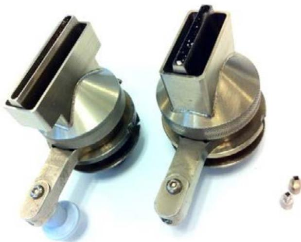
Figure 15: Large site cleaning nozzle (Zevac AG).
