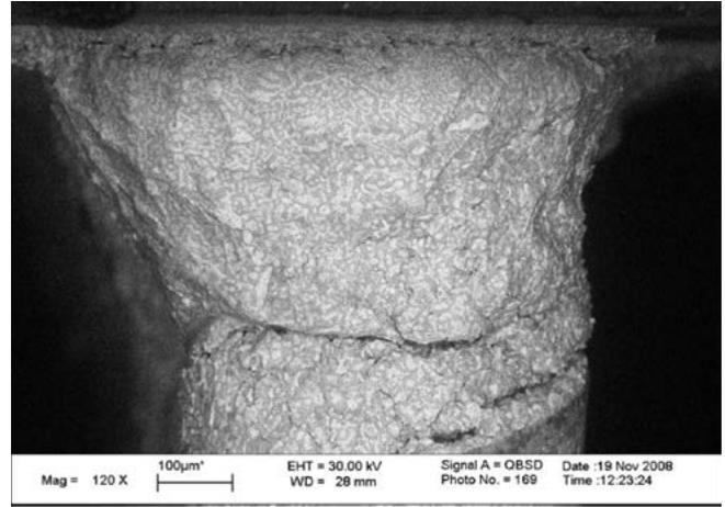
Figure 10: SEM photomicrograph of re-columned and reassembled CGA560 after thermal cycles and prior to X-sectioning showing different types of microcracks in column and solder at the package side.
