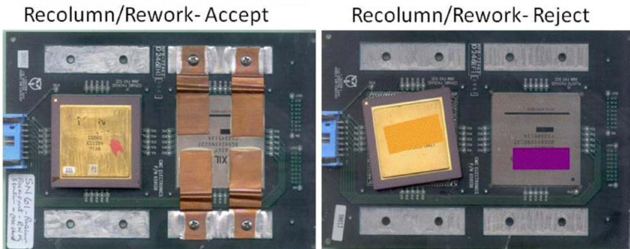
Figure 4: Representative TVs after re-assembly of re-columned CGA560 packages: one with acceptable quality and the other rejected with gross package twisting occurred during solder reflow by a rework station.
