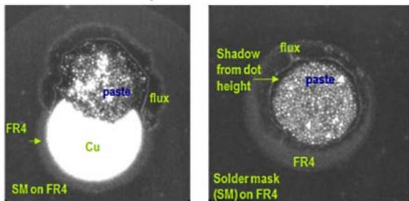
Figure 3: Factors to take into account for correct recognition.
