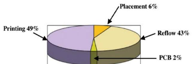
Figure 6: Root cause of defect.
