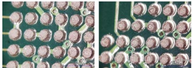
Figure 15: Optical photomicrograph of paste deposition with mini-stencil with acceptable solder paste quality (left) and reject (right).
