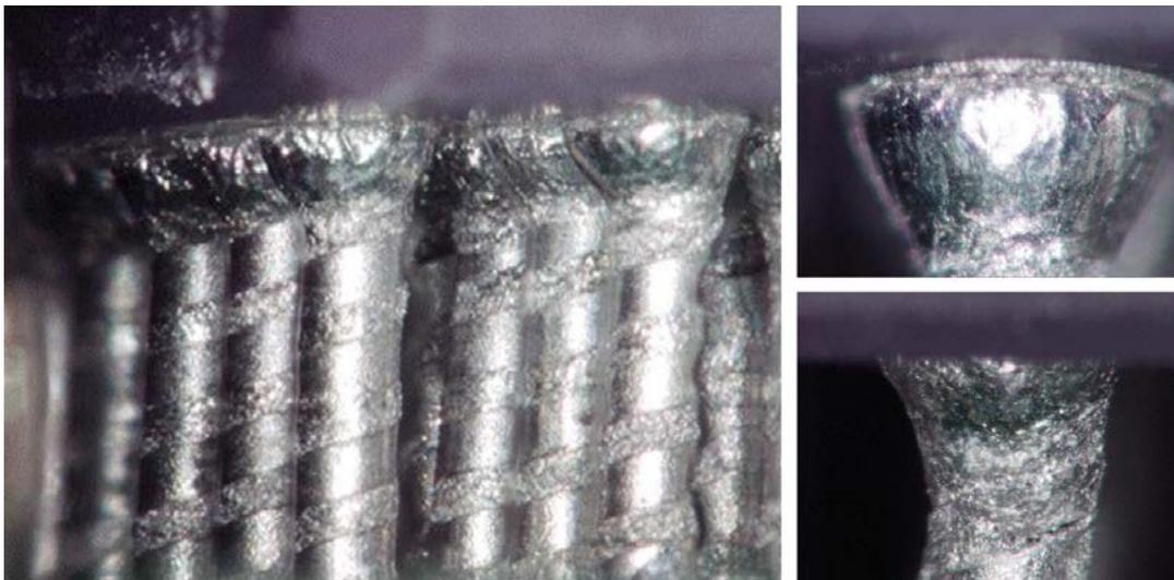
Figure 19: Representative optical photomicrographs, including those with pseudo 3-D optical photomicrograph, showing damage and microcracks at the package side.
