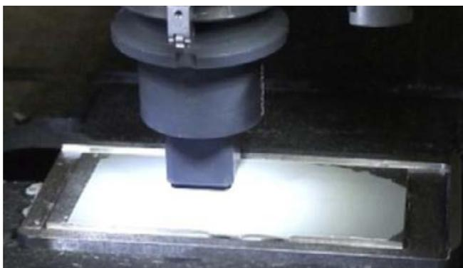
Figure 16: Force-controlled solder paste dipping.
