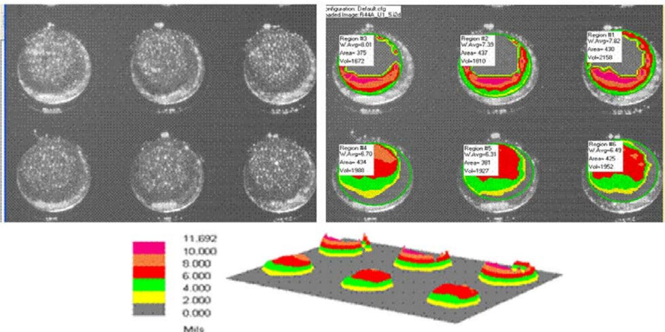
Figure 16: Optical photomicrograph and measured/calculated solder paste information for paste print with ministencil with 7-mil thickness and 23-mil aperture opening diameter.
