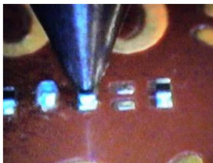
Figure 8: 01005 Micro-tip nozzle.
