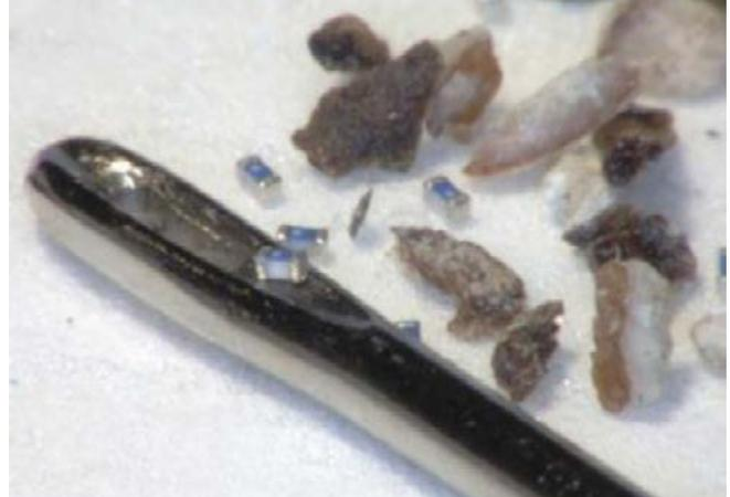
Figure 5: 01005 in eye of needle and next to pepper flakes.
