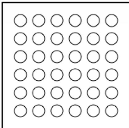
Figure 27a: 1.00 mm diameter circles @ 1.2 mm pitch—50% coverage<sup>[10]</sup>.
