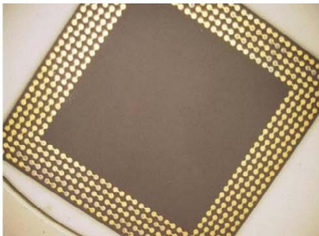
Figure 2: Optical photomicrographs of a removed CGA560 package after rework showing removed/shorted columns (left) and package daisy chain pattern without interposer (right).
