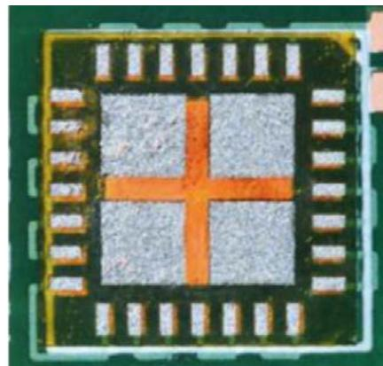
Figure 25c: Stay-in-place site stencil<sup>[8]</sup>.
