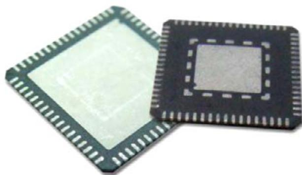
Figure 23: QFN/MLF devices.
