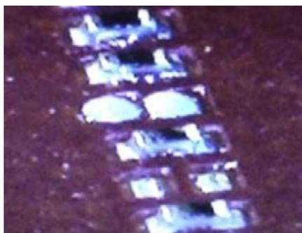
Figure 9: Paste transfer onto 01005 pads.
