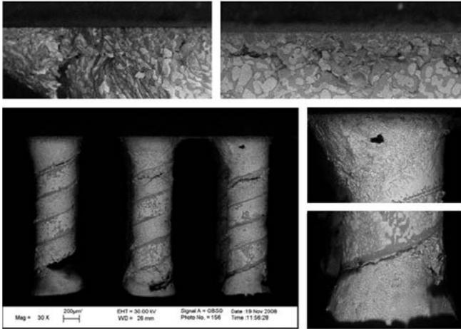
Figure 9: SEM photomicrographs of re-columned and reassembled CGA560 after thermal cycles and prior to X-sectioning showing microcracks in columns and solders at the package side.
