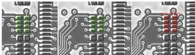
Figure 4: Paste offset—place on CAD coordinates, paste location or disallow.
