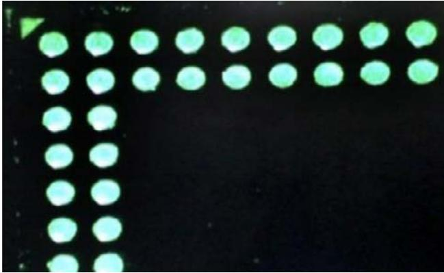
Figure 18: Inspecting paste on spheres in vision.
