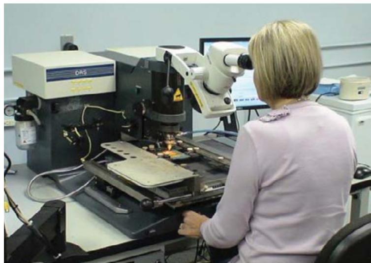
Figure 7: Man/machine 01005 rework interface (MMRI).
