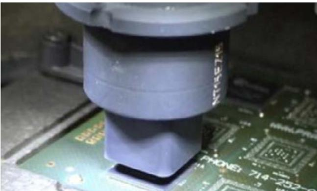
Figure 12: Standard nozzle removes one package at a time.
