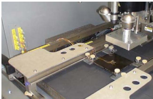
Figure 1: Instrumented 114 mm BGA on BGA rework system.
