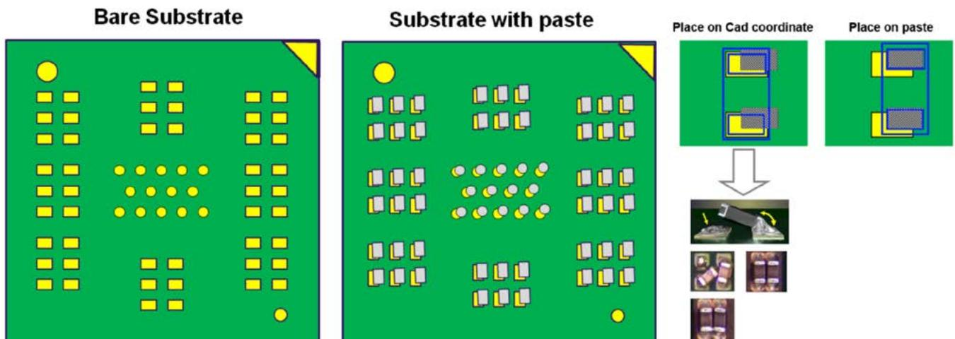
Figure 1: When placing on CAD coordinates, paste offset may lead to defects.
