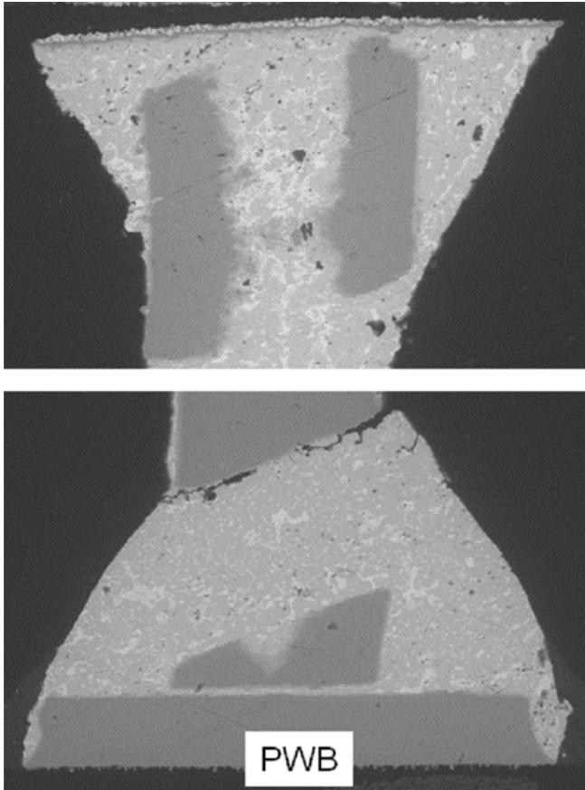
Figure 12: X-section photomicrograph of re-columned and reassembled CGA560 after thermal cycling showing interfacial condition at package and PCB sides. Full cracking at the package side is apparent.
