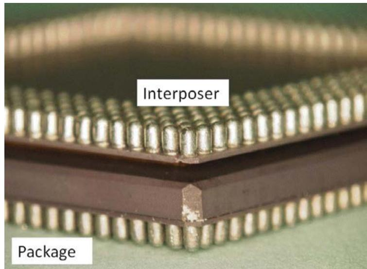
Figure 1: Optical photomicrograph of a virgin CGA 560 I/O package before re-columning with interposer (bottom) and an interposer layer alone on the top.
