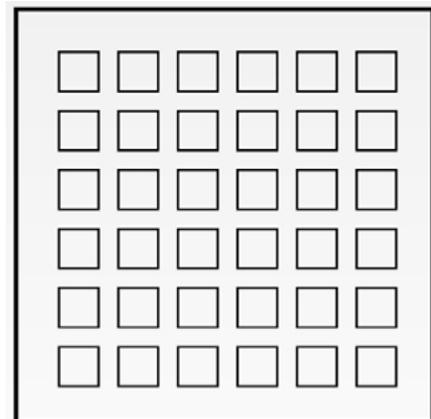
Figure 27c: 1.35 x 1.35 mm squares (10) @ 1.5 mm pitch—81% coverage<sup>[10]</sup>.
