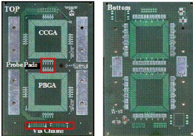
Figure 3: PCB design showing package daisy chain, probing pads, and via daisy chains.
