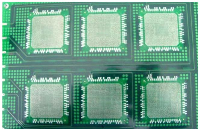
Figure 14: Optical photo of a high I/O CCGA board after paste printing with a ministencil.
