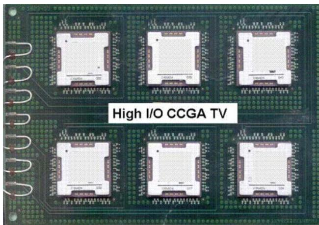
Figure 18: Photograph of an assembled test vehicle having six re-columned, high I/O CGA packages.
