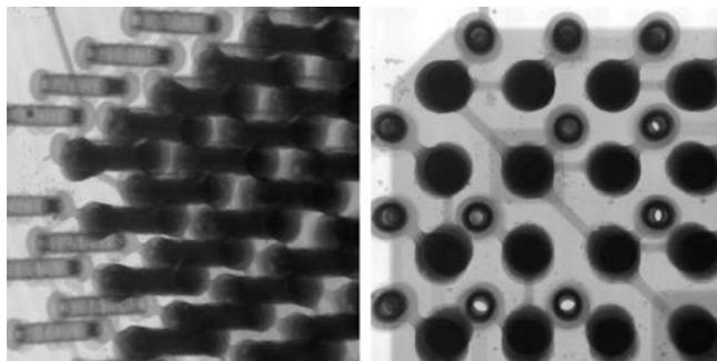
Figure 6: X-ray photomicrographs for re-columned and re-assembled CGA560 after thermal cycle exposure showing solder balls, but no separation at package pads detected visually.
