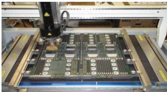
Figure 3: 22 x 24 high-thermal-mass PCB on large board rework system (board courtesy of IBM).
