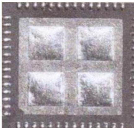
Figure 25b: Bumped QFN after reflow and removal of stencil<sup>[8]</sup>.
