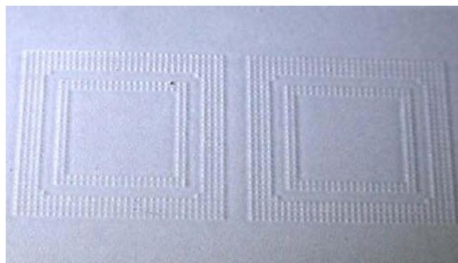
Figure 17: Multiple imprints in solder paste.
