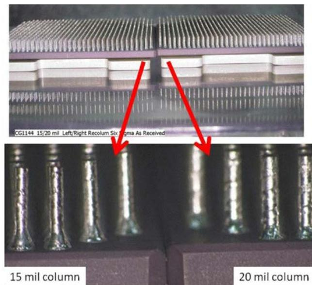
Figure 13: Photomicrographs of the two sizes of re-columned packages (20- and 15-mil columns) at low and high magnifications.
