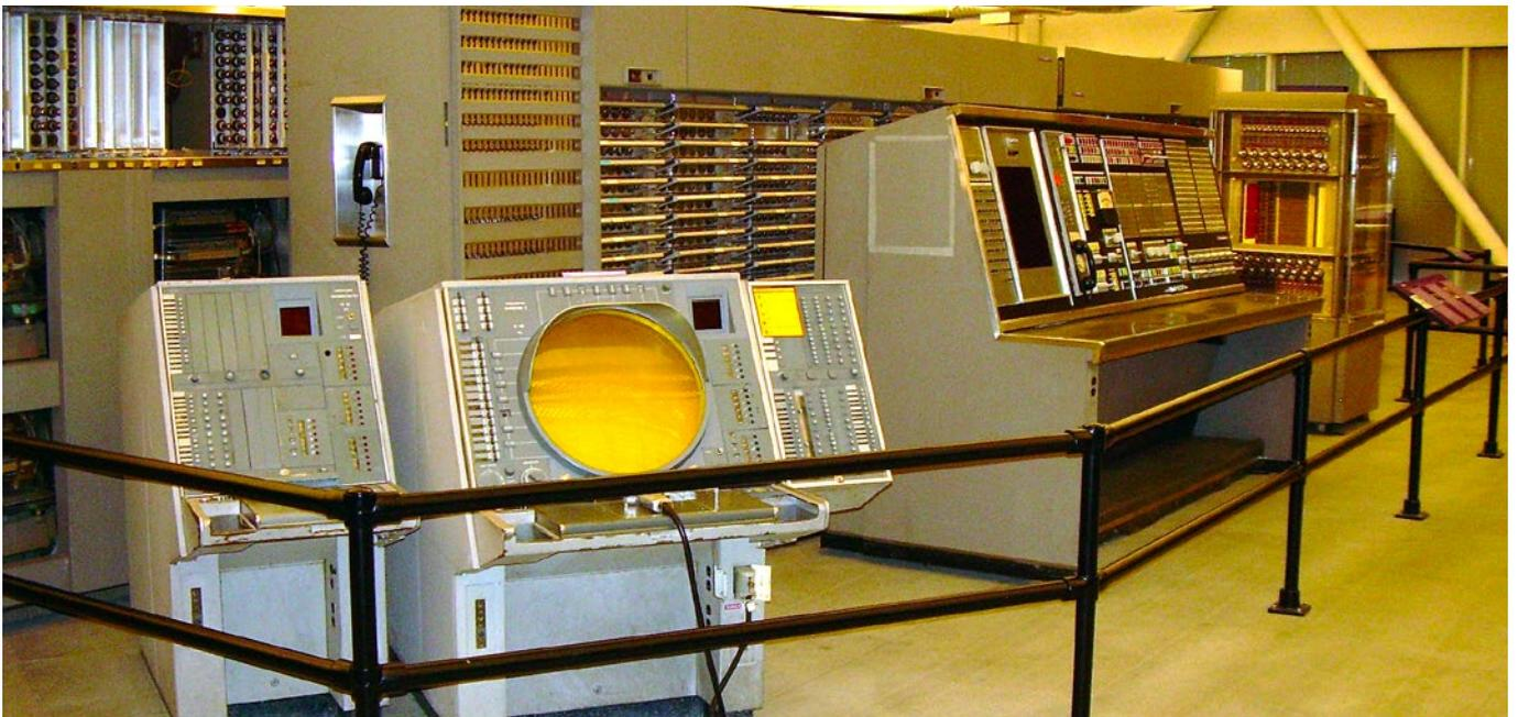
Figure 5: All the elements of a SAGE computer system and consoles. The 20-inch OA-1008 Situation Display (SD) shown in the forefront was equipped with a light gun for a user interface. As Air Force personnel would man the console in eight-hour shifts around the clock, perhaps that is why the console was equipped with a cigarette lighter and ash tray! (Image: Steve Jurvetson, Wikimedia Commons)
