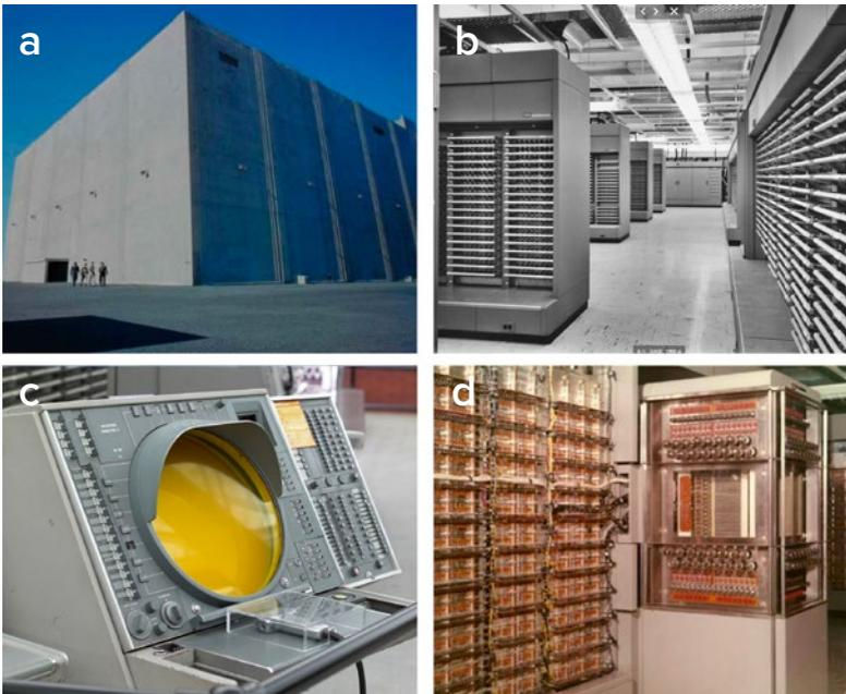
Figure 4: A SAGE system: a) CC/DC blockhouse; b) the SAGE tube-based computer; c) The circular CRT display screen; d) the 256 KB core RAM.<sup>7</sup>
