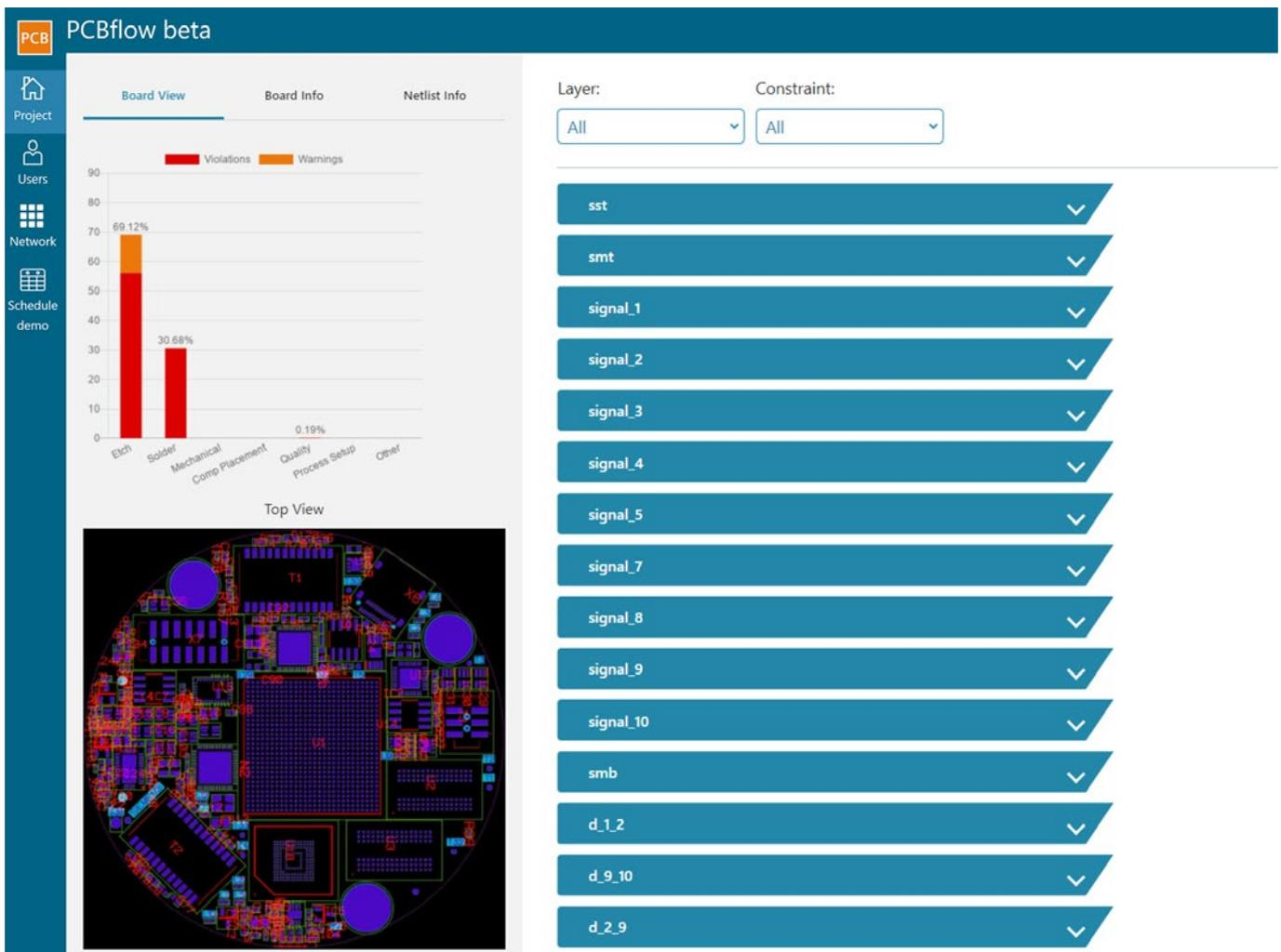
Figure 2: DFM report with information pane (left) and analysis results per layer (right).
