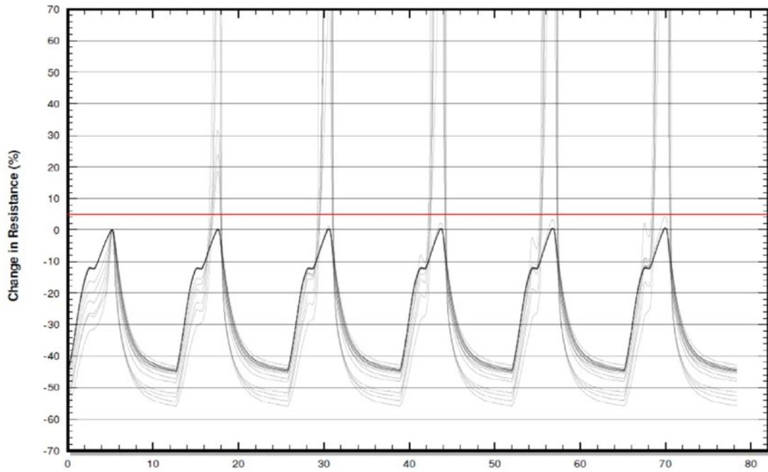
Figure 18: Resistance during the reflow of Net1 (notice that all coupons pass the first cycle).
