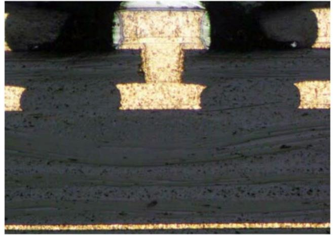
Figure 16: A microvia at 0.005" with an aspect ratio of 1:1 and a dielectric target of 0.0045".
