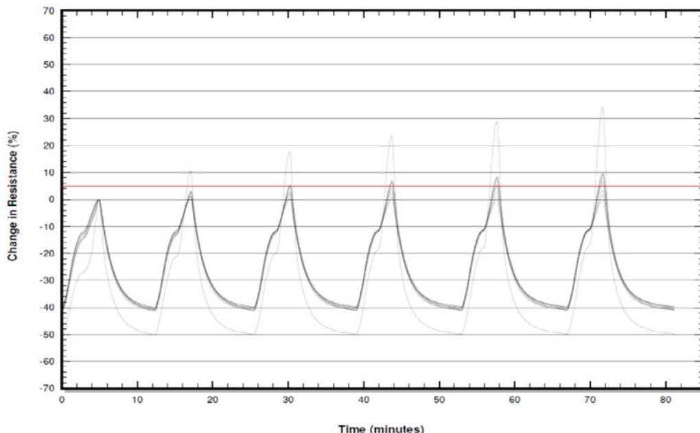
Figure 9: OM testing with four-wire resistance from ambient to reflow temperatures.
