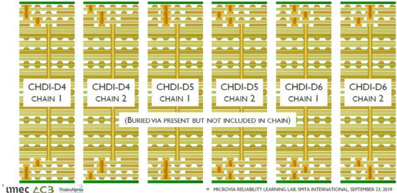
Figure 8: The modified ESA microvia test panel for the IPC reliability testing using the Hitachi high-Tg laminate. (Source: IMEC)
