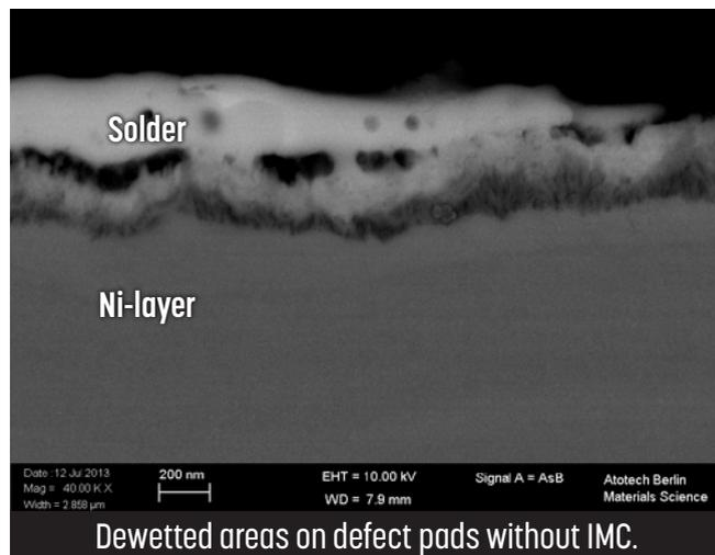
Figure 3: Exemplary SEM images of defect pads in a cross-section.
