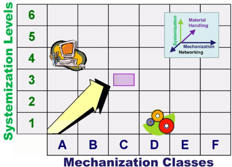
Figure 1: The automation vector is defined as systemization and mechanization, including material handling and networking between work centers.
