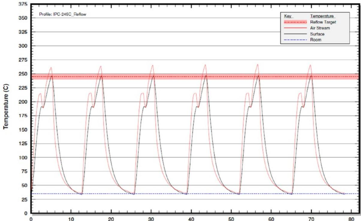
Figure 17: OM thermal cycling on the actual D-Coupons.
