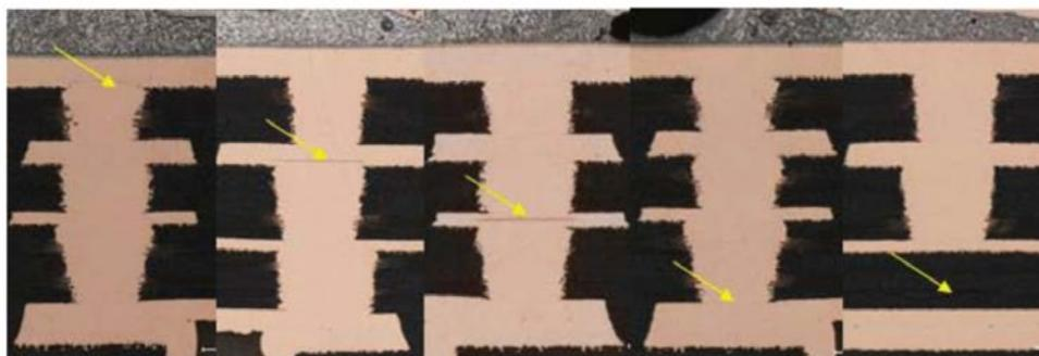
Microvia “partial” fractures found throughout stacked electroless Cu interfaces, as well as within the laminate resin, which indicates CTE-z stresses essentially the same at all levels.
