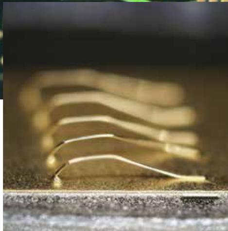
**Pic. 1:** Applicable for Au-wire bonding on ENEPIG
