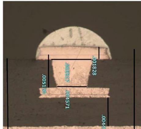
Figure 20: Remake with correct via and dielectric.
