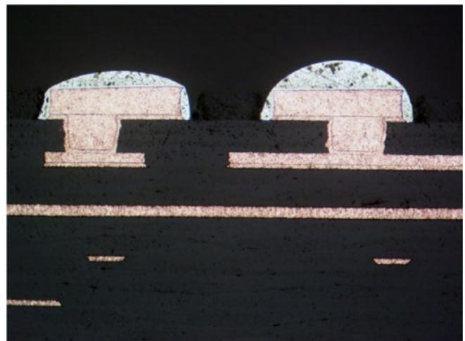
Figure 4: Micro-etched cross-sections hide small separations found in the polished condition.
