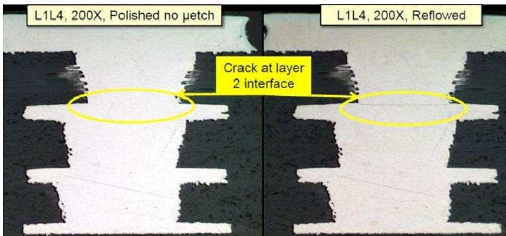
Figure 2: Two microvia stacked constructions with the typical microsection on the left, where the problem is invisible, compared with after reflowing, where it is almost invisible. (Source: Motorola Solutions)
