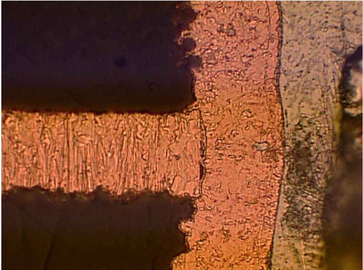
Figure 2: Type 1 ICD.
