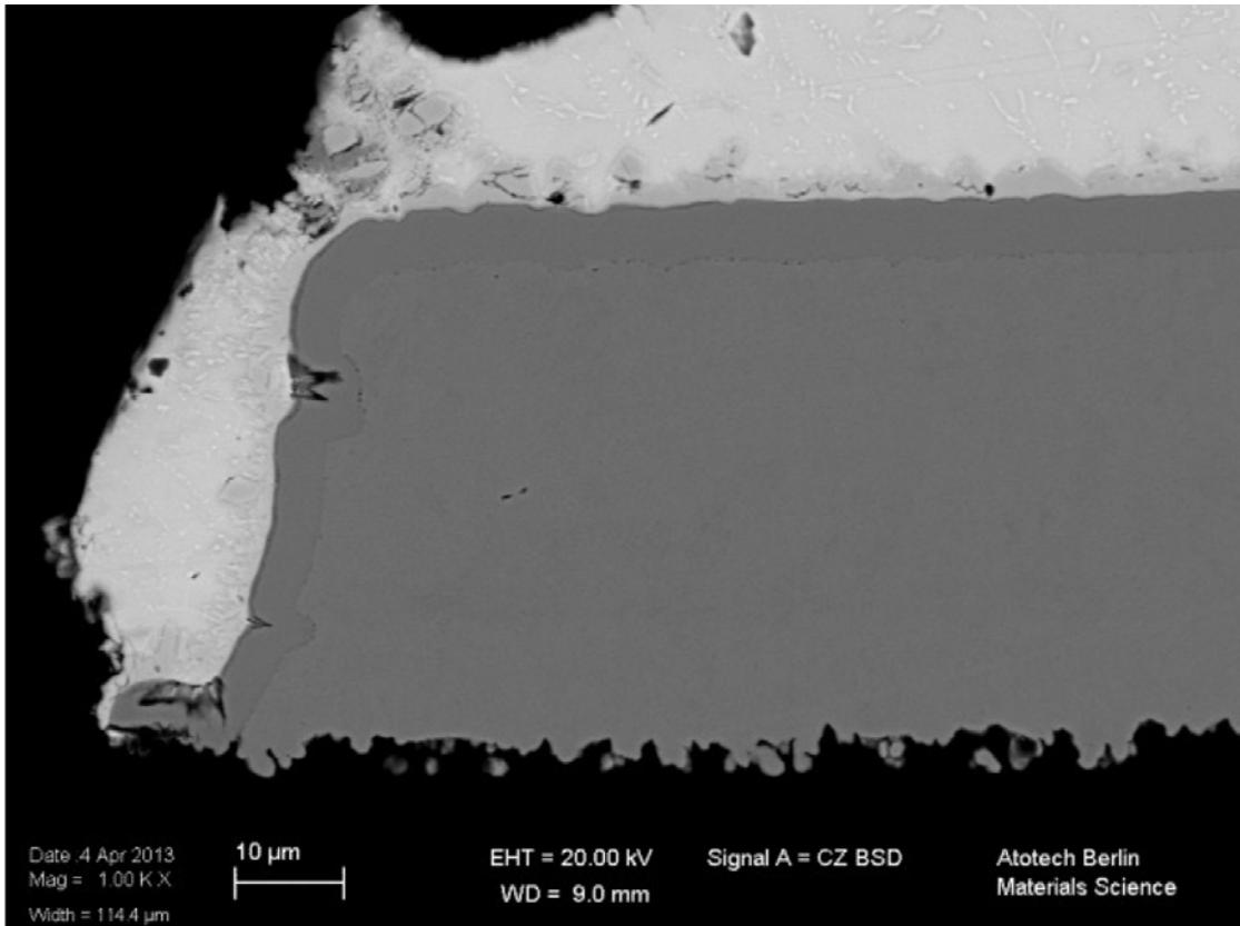
Figure 4: IMC formation at a single corrosion location on a soldered pad.
