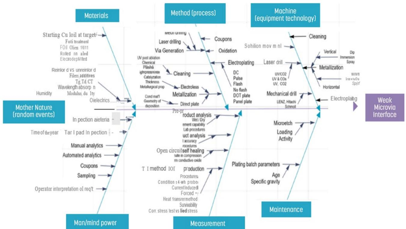
Figure 5: Various factors in the understanding of weak interfacial bonds for microvias.
