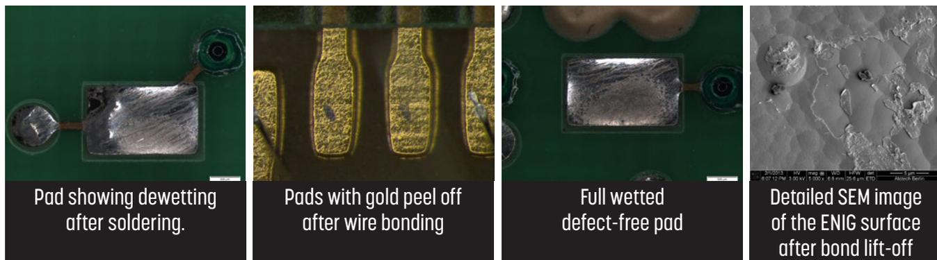
Figure 2: Exemplary pictures of failure modes of ENIG finishes in soldering and bonding.
